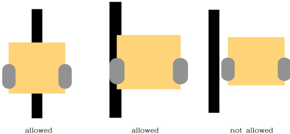
3.2 If the robot's controller (both wheels) crosses the black line, it is considered off the track.
